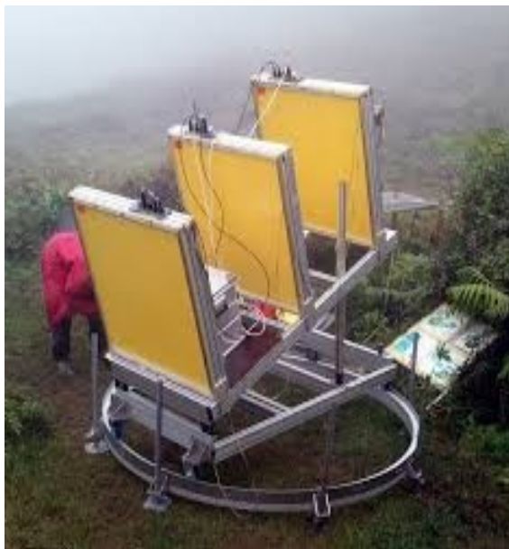
Figure 4: Analyzing the internal structure of a volcanic zone using muons
